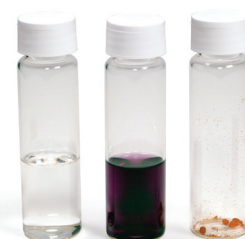
Figure 9. Left to right: CBD before Beam test; HU-331 after Beam test; crystalline HU-331.
