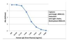
Sandwich ELISA using IgE (human) Rabbit Monoclonal Antibody - Biotinylated as the capture antibody (25sg/well) and Ig Light Chain (human) Rabbit Monoclonal Antibody - Biotinylated (Item No. 32112) as the detection antibody, followed by an alkaline phosphatase-conjugated streptarvidin.
